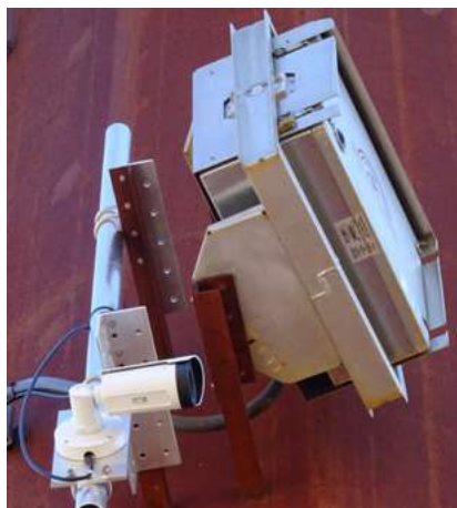
Figure 86. Smart vision cameras installed on a transmission tower to monitor collisions. © James F. Dwyer and Richard E. Harness
