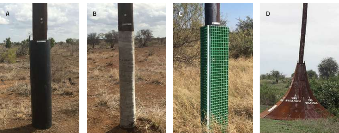
Figure 187. The four mitigation products tested to limit/prevent contact between wildlife and poles in the Kruger National Park: A: Steel pole sleeve; B: Polefix industrial cast; C: FRP Grating box; D: VB Rhino. ©Endangered Wildlife Trust
