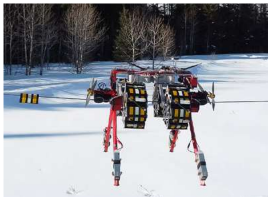
Figures 78 and 79. Helicopter installation of line markers (left). The UAS-deployed Linefly line marker installation robot (Fulcrum Air, Calgary AB) (right). ©EDM International, Inc. (left) and James F. Dwyer and Richard E. Harness (right)
